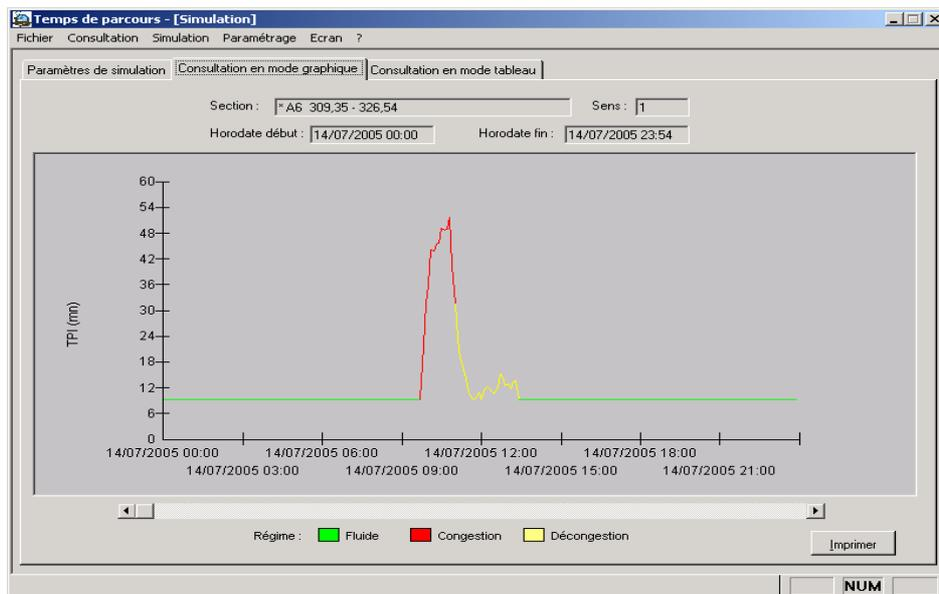
**Figure 4 – An example of TPI screen during an accident**
