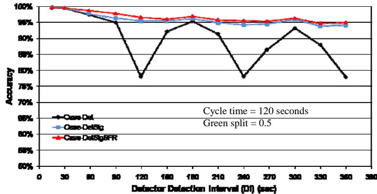
Figure 5: Detector detection interval versus accuracy.
