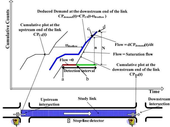
Figure 4: Flow pattern at downstream end of the link for case-DetSigSFR.
